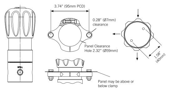
Regulator height: 7.4" (188mm) Body Diameter: 2.44" (Ø62mm)
